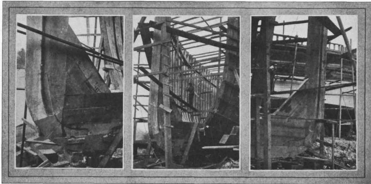
FIG. 91—DETAILS OF FOREFOOT SHOWING USE OF NATURAL KNEE AND ANGLE BLOCKS. FIG. 92—ANOTHER VIEW OF THE SAME STEM. FIG. 93—SAME STEM FROM THE OPPOSITE SIDE
